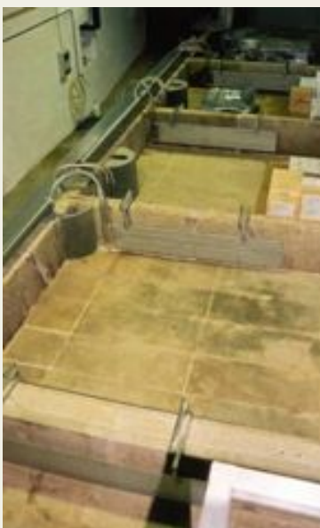
Three types of fermenter. On the left we have a lagar (this is a swanky one with a heat exchanger), ideal for shallow fermentation with good contact between the juice and skins. Traditionally, these are foot-trodden, and this one hails from Portugal's Douro.
