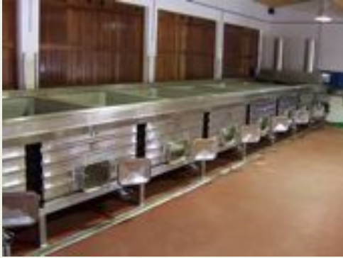
Above we have a row of open-top fermenters, which are quite small and ideal for processing high-quality red wines (again, this is from a winery in Portugal, this time the Alentejo). Then there is a rotary fermenter of the type popular in Australia.
