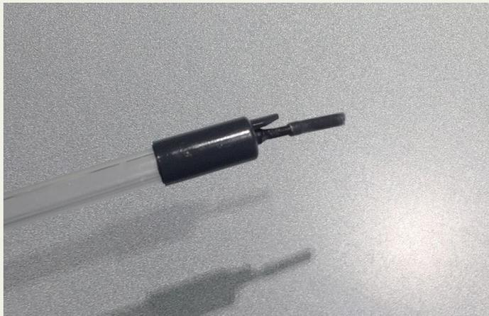
**Editor - If you are having problems with your bottle filler tip sometimes not depressing in some, deep or tight punt bottles, extend the tip with a small piece of tubing. I think this tubing was a piece of wire insulation. ...**
