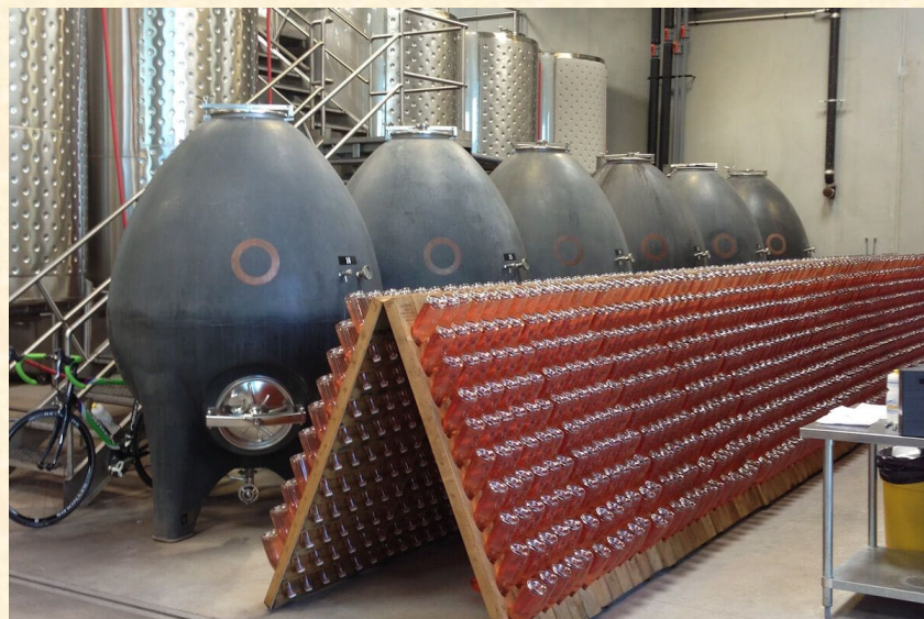
Egg shaped fermenters at the Okanagan Crush Pad winery in British Columbia
