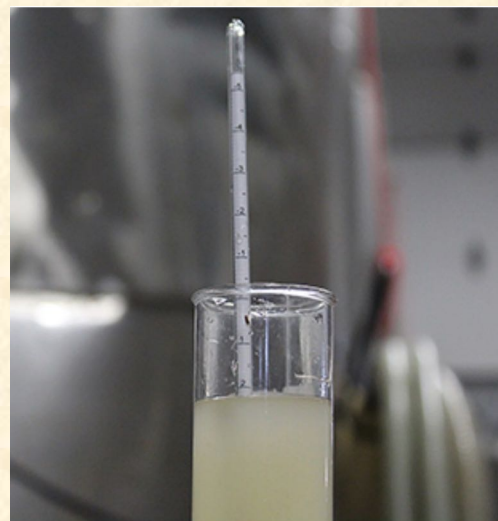
A precision hydrometer is critical to accurately measure the gravity of the fermenting wine so that it can be bottled at just the right gravity to result in the desired level of carbonation and residual sugar.
