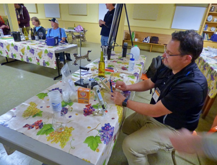
Rob Marr set up to measure SO 2 in a wine sample using his Vinmetrica 300. This instrument can also measure MLF, pH/TA, ABV, residual sugar, DO, and YAN as well as other tests.
