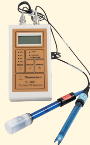
Rob Marr set up to measure SO 2 in a wine sample using his Vinmetrica 300. This instrument can also measure MLF, pH/TA, ABV, residual sugar, DO, and YAN as well as other tests.
